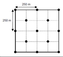
• = wind power station tower Note: Drawing is not to scale.
